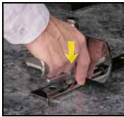
Place the Bier Pin in one of the hexagonally-shaped holes.
