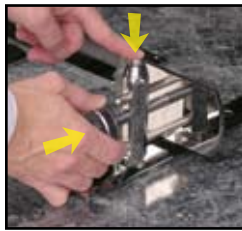
Depress the top button and push the knob until the Bier plate is close to the casket or Commemorative Carriage.
