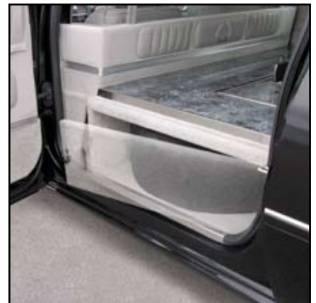
Full-sized spare tire storage compartment under the floor on the driver's side.
