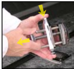
Depressing the top button releases the tightening knob and shaft to fully open the Bier Pin.
